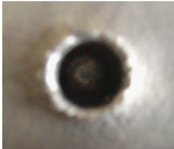
Fig. 11. Photo of a crater made by the lead bullet imbedded into a lead plate. Inside of the crater the remains of the bullet can be seen.
